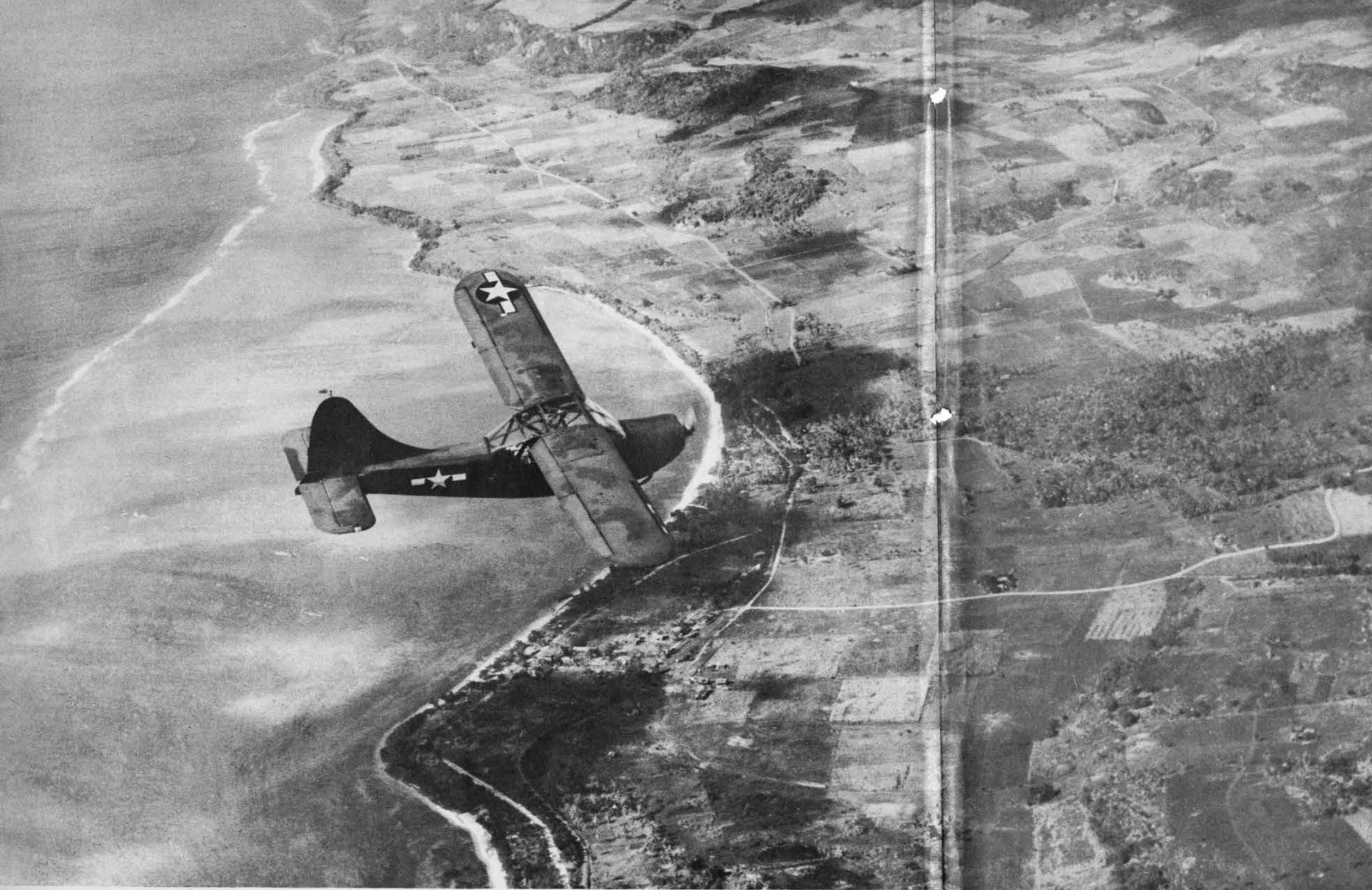
L-5, NEWEST ARMY OBSERVATION PLANE, DIRECTS NAVAL GUNFIRE AGAINST SAIPAN. TRANSPARENT COCKPIT OPENS THROUGH WING, PROVIDES GOOD VISIBILITY. TAILPLANE AND WING ARE RECTANGULAR WITH ROUNDED TIPS
